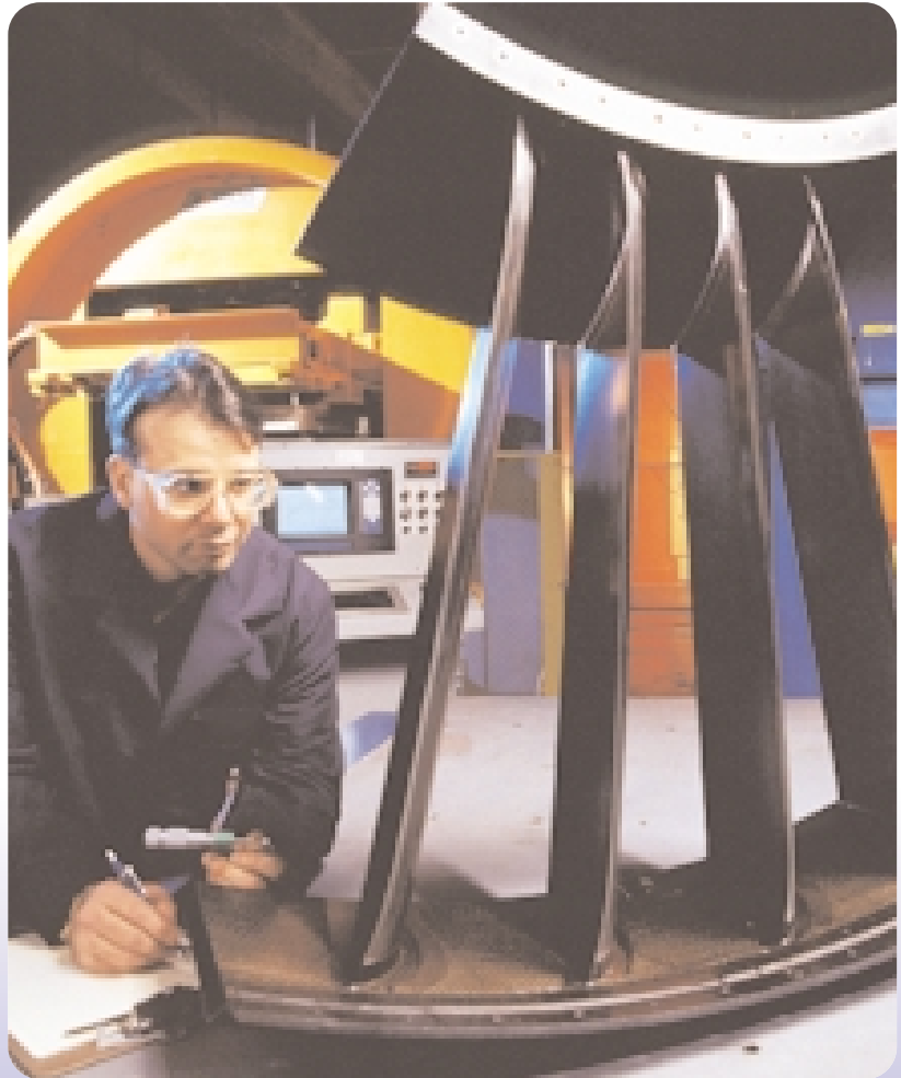
Turbo Fan Exit Case. One piece AdvRTM molding. Ten of these complex units combine to replace a traditional titanium assembly.
