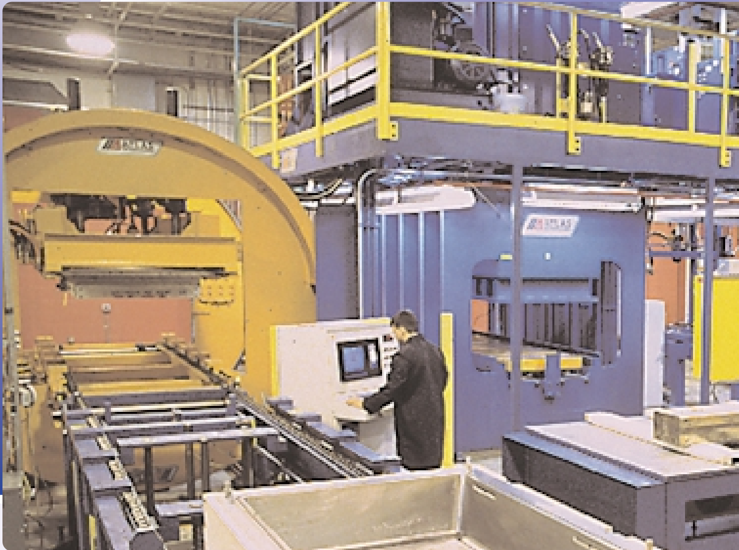
Flexible Molding Cell. Computer management of cell scheduling, tool handling, thermal cycle and resin injection.
