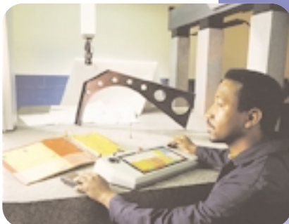
Coordinate Measuring Machine is used to assure conformance of parts to the electronic master.
