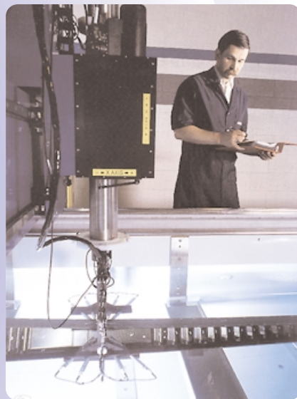
Quality evaluation may involve advanced ultrasonic inspection.
